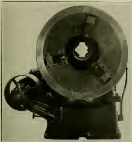
REAR VIEW SHOWING CHUCKS OF THE LANDIS PIPE CUTTING AND THREADING MACHINE.
